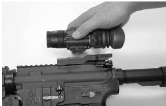
Figure 3-3 Attaching ATN NVM-14 to Weapon Mount
